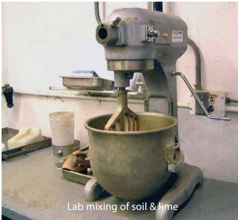
**Procedure:** Make a mixture of soil, lime, and water at the minimum percentage of lime as determined from Step 2 (Eades-Grim test), using a water content of OMC + 2-3%. Seal the mixture in an airtight, moisture proof bag stored at room temperature for 1-24 hours. Determine the OMC and MDD of the mixture using ASTM D 698 procedures (standard compaction effort) [16].
