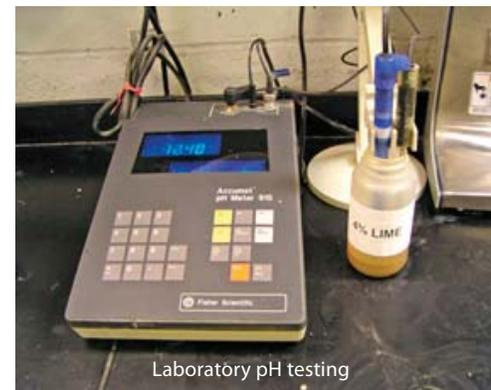
**Criteria:** The lowest percentage of lime in soil that produces a laboratory pH of 12.4 [flat section of the pH vs. lime percentage curve produced by the test] is the minimum lime percentage for stabilizing the soil.
