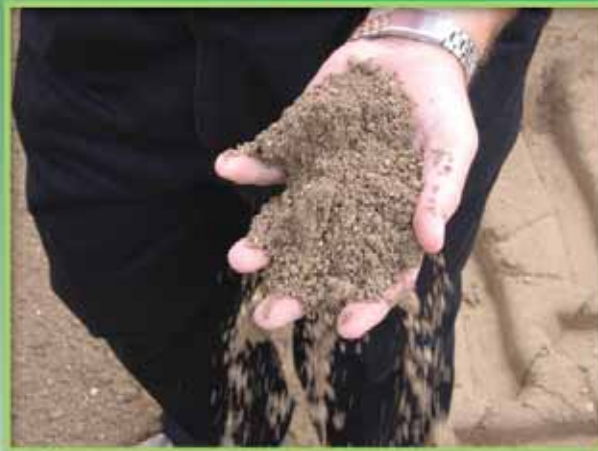
Soil After Lime Stabilization
